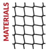
Using N820BK is knotless netting with a 21/2 inch square mesh. Knots are eliminated using a balanced knitted construction with filaments running continuously throughout the netting to enhance strength and durability.
